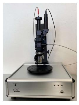
**FR-Scanner-AllinOne-Mic-XY200** is the modular platform that integrates under the same roof state-of-the-art optical, electronic, and mechanical modules for the characterization of patterned thin and thick films. Typical examples include (but are not limited to): micro-patterned surfaces, rough surfaces, and numerous others.
